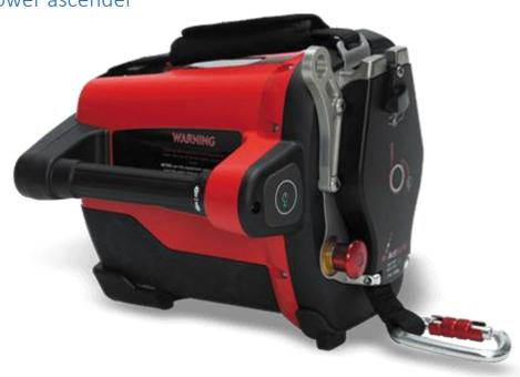
The ACX Ascender features a closed self-locking rope grab, a distinct battery management system and an IP55 protection. The left-hand bi-directional throttle and the remote control reaching up to 150 metres are some of the many aspects that make the ACX Power Ascender safe and easy to use. The ACX Power Ascender is the latest model of ultra-portable battery-powered ascenders. This Device can work smoothly and safely in most places, high or low, confined or remote.
