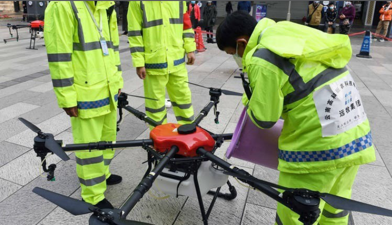
Workers in Kunming City, Yunnan Province, China refill a drone with disinfectant. The city is using drones to spray disinfectant in some public areas. Image: Xinhua News Agency/Yang Zongyou via Getty Images
