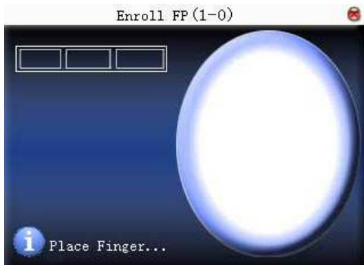
Press finger according to device’s prompt. Press the finger, three times in the proper way.
